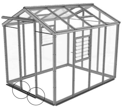
Now install the bottom door guide, start by fitting the door cill, diagram 35. Attach the cill to the base sections using the small plate (HE512M) and two 10mm nuts and bolts. (Keep this bracket as close to the ground as possible so it doesn't interfere with the threshold strip).
