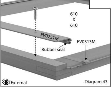
When in position you can fix the glass in place with the vent capping (either cedar or aluminium) using the 25mm screws, diagram 43. Remember if you are using the aluminium capping system you will need to insert the rubber seal before fixing it in place.
