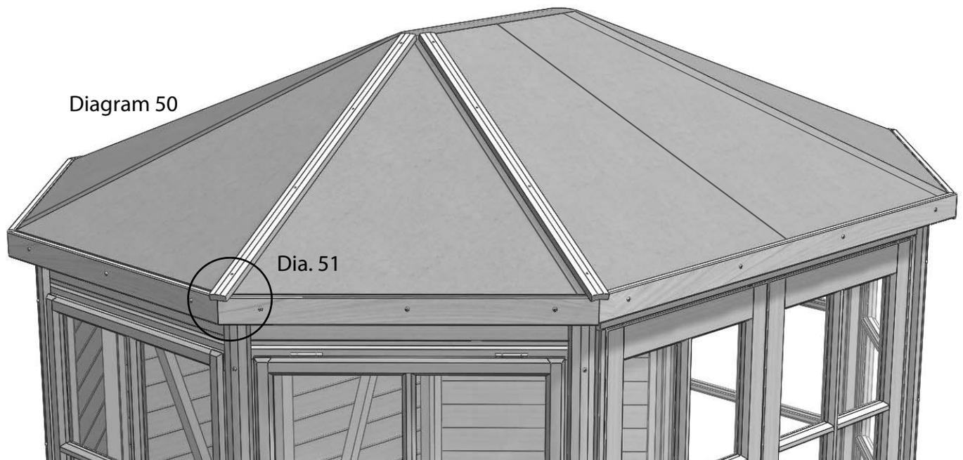
Now you can fit the capping working your way around the building. As you position each one, line the end up with the outer point of the joint between fascias (diagram 51). When you are happy fix in position with 50mm countersunk stainless steel screws. Only fix the bottom screw for now as you will want to fix the top screw next, when all have been spaced equally.
