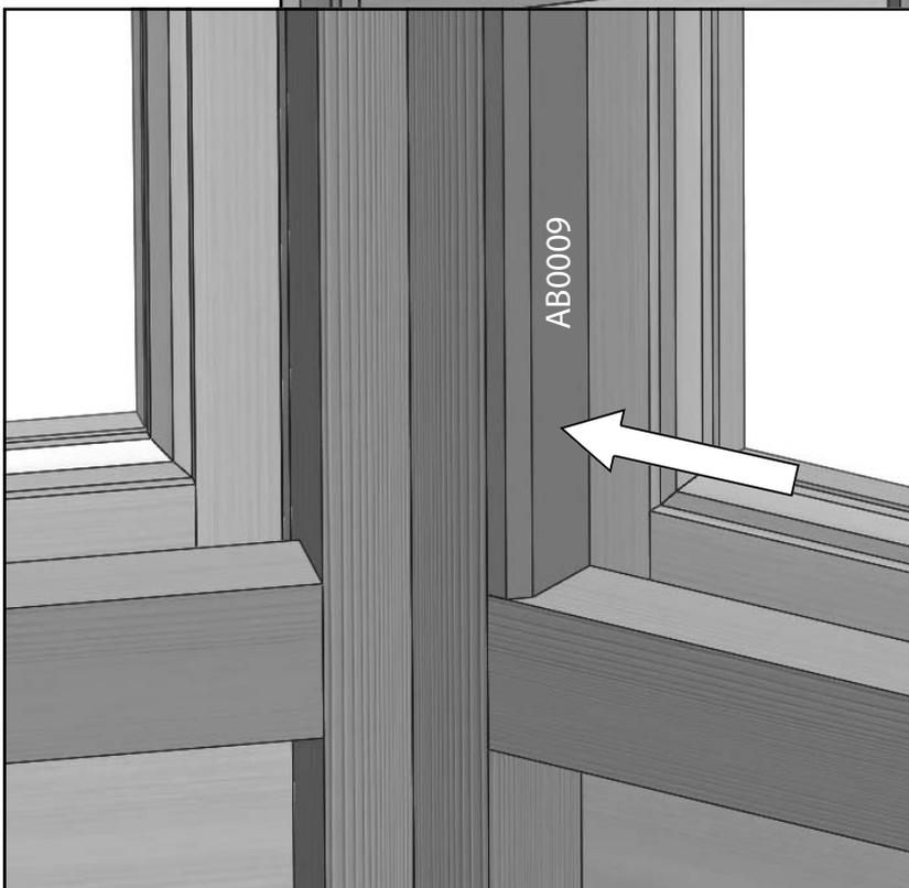
As with the architrave the window trims are fitted with four panel pins per side. (diagram 74). These need to be fitted to all window sections.
