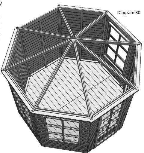
With all the roof bars fixed in place you can attach the ply roof sheets. Use  $1^{1/2}$  inch countersunk screws to fix this. You should have 4 down each side with one in the middle at the bottom. Use the grove in the roof bars to help you line up the roof sheets (diagram 32).
