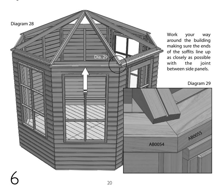
Its best to fit all the soffits to the sides leaving the last one in the least visible place possible in case you have to trim the soffit or there is a slightly larger gap than normal.
