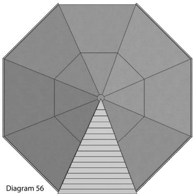
Fit each fascia to the building leaving the one that is least visible to last in case it needs trimming or there is a slightly bigger gap. All being well it should slot in nicely.
