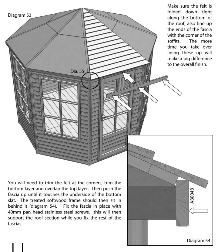
When fitting the next fascia board adjust the position until you get a neat joint between the two boards. You may find you need to adjust the first one to get them to sit correctly. You will need to trim the felt at the corners, trim the bottom layer and overlap the top layer.
