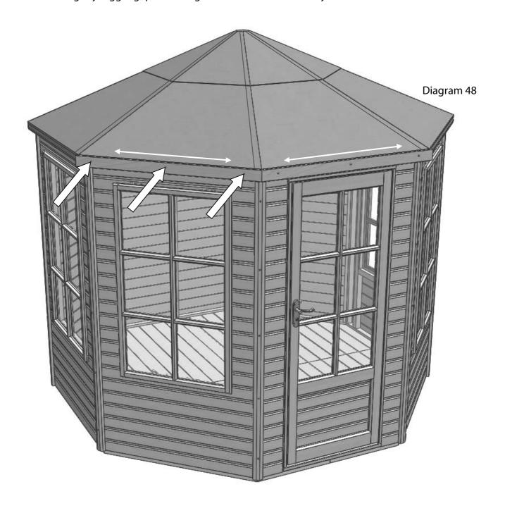
Before you can fix the roof capping in place you need to trim it to length (the full length capping is used on the optional slatted roof). Trim the end with the bevel so the square end that goes at the bottom of the roof is kept tidy and pre-treated. **DO NOT CUT THESE IF YOU HAVE A SLATTED ROOF**
