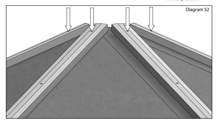
Finish fixing the capping with the final 2 screws per strip. Once fixed in place you can trim any excess felt. Be very careful not to cut through both layers of roof felt. Scoring down the side of the capping a couple of times lightly is much safer than trying to cut through in one go!
