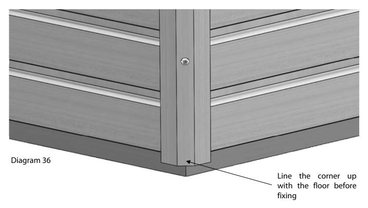
You can now fix the sides to the floor. Drill pilot holes in the cill section of the side frame and fix
