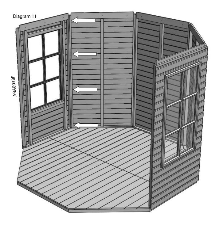
Fitting the next panel requires a slightly different approach as you can't simply drill and screw through at right angles to the frame. You need to get the drill in as close as you can and drill at an angle through side of the frame.
