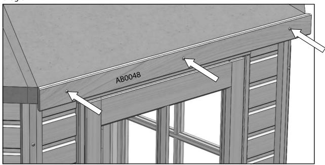
When fitting the next fascia section adjust the position until you get a neat joint between the two sections. You may find you need to adjust the first one to get them to sit right. Measure from the underside of the soffit to get the fascia in the same position as the first.
