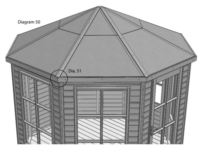
Now you can fit the capping working your way around the building. As you position each one, line the end up with the outer point of the joint between fascias (diagram 51). When you are happy fix in position with 50mm countersunk stainless steel screws. Only fix the bottom screw for now as you will want to fix the top screw next, when all have been spaced equally.
