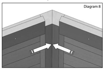
When fixing the panels bear in mind which faces will be most visible when you walk into the building. Try to keep the screw heads on the least visible faces where possible.
