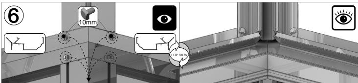
IMPORTANT: Because your porch gutter sections are welded together to eliminate the chance of any leaks the holes circled above can vary slightly in their locations. They may therefore require slight alteration to marry up with DV363 and DV381. Using an 8mm drill bit to enlarge the standard 7mm holes will for example give a little more play to aid fitting.
